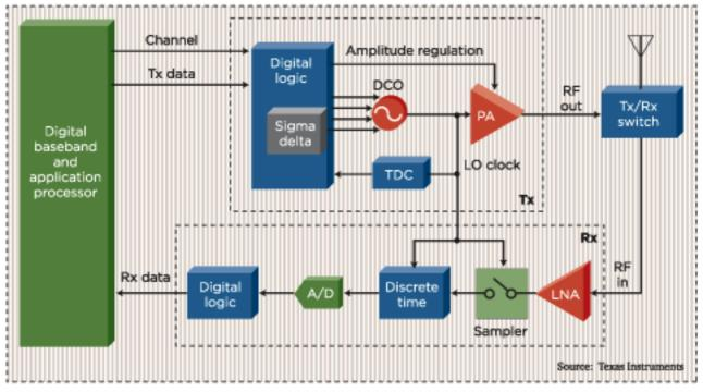
**To leverage** fully the attributes of a deep-submicron CMOS process, a novel transceiver architecture has been demonstrated that comprises an all-digital frequency synthesizer and transmitter as well as a digitally intensive discrete-time receiver.
